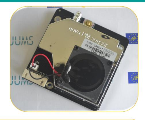
The Nova Fitness SDS011 is a low cost particle counter. It is based on the light-scattering principle and can detect particles form 0.3 up to 10  $\mu m$ . The number and diameter of particles can be obtained by analysis because the signal waveform has certain relations with the particles diameter. This sensor is often used in citizen science projects.
